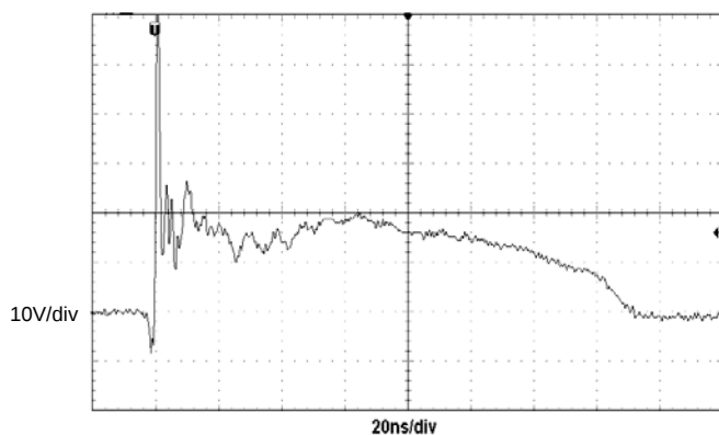
ESD clamping (+8kV contact discharge per IEC61000-4-2)
